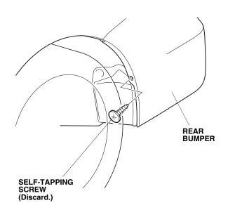
Secure the left rear splash guard using two 5 x 25 mm self-tapping screws tightened in the order shown.
