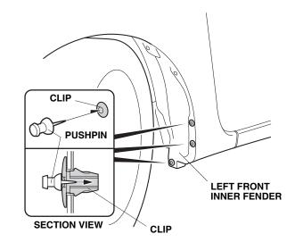
2. Using a pushpin, pierce the center of the three clips on the left front inner fender.
